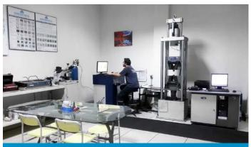
Metallurgical Laboratory with Spectrometer, Hardness, Tensile Strength and Impact Test Devices
