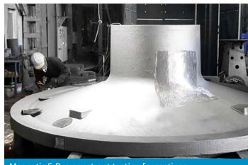
Magnetic & Dye penetrant testing for castings
