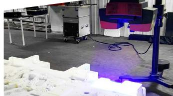
ATOS 3D Scanning and Measuring System for dimensional control of patterns and castings
